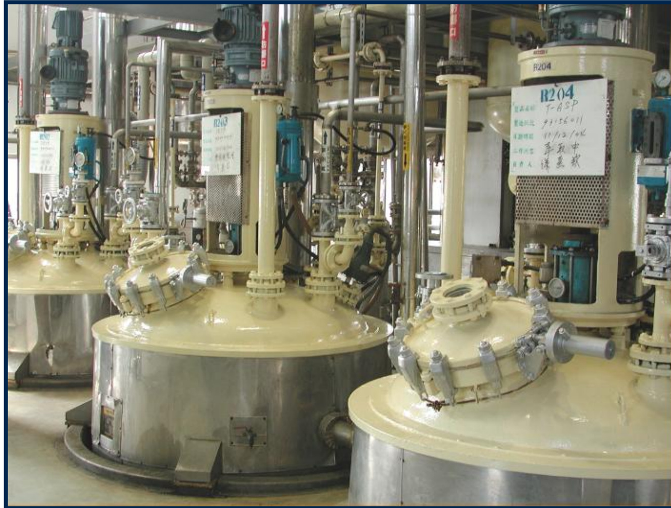
3,000 L Glass Lined Reactors
